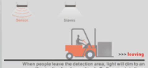
The sensor automatically switches on light when motion detected.
