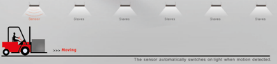
When people leave the detection area, light will dim to an illumination level preset and off after a certain time.
